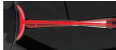
Fig 3. A cast image or shadow created by the contaminant in the oil creates a measurable change in the light intensity.
